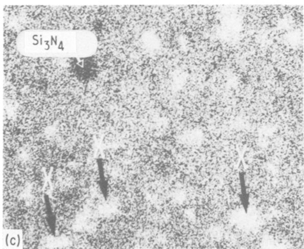
Figure 11 Detection of the 12H Sialon polytype with the EPMA: (a) SEM micrograph of Grade 3; (b) cathodoluminescence micrograph with detector set to image total emitted light; (c) aluminium X-ray map of same area. The 12H Sialon particles are marked X.
